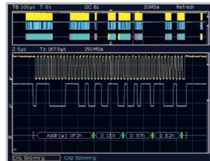
I<sup>2</sup>C Bus Hex Decoding on the Analog Channel
